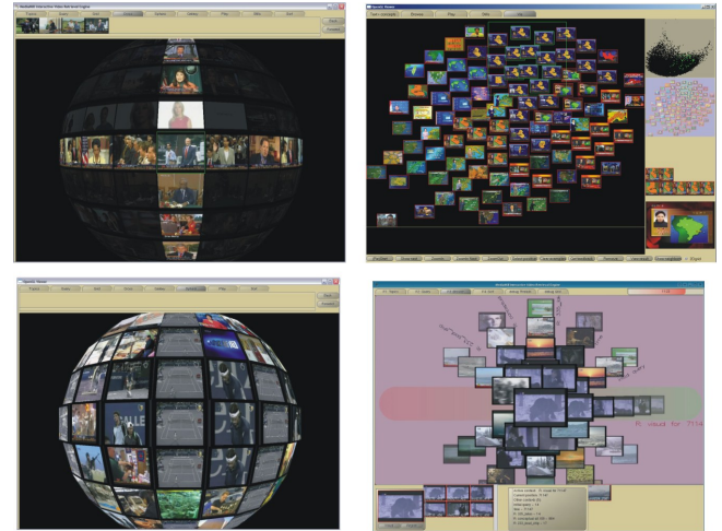
Fig. 2. Browsers in the MediaMill search engine. Top left the CrossBrowser (showing a ranked query result vertically and the timeline of the program horizontally), bottom left the SphereBrowser (with a tennis thread in the center), top right the GalaxyBrowser (several clusters of different maps visible) and bottom right the RotorBrowser (showing several threads containing the current shot).
