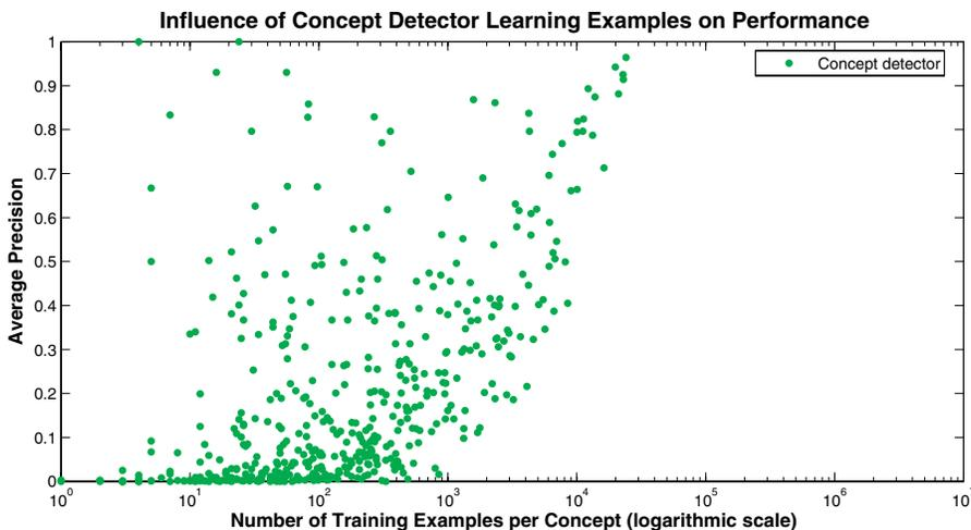
Fig. 4.3 Detection results [219] for a lexicon [163, 230] of approximately 500 concepts on TRECVID 2006 video data. Good performance is obtained for detectors of concepts with limited variability in their visual appearance, such as broadcast news specific concepts, and concept detectors which are trained on many examples like *face* and *outdoor*. Most concept detectors perform moderately because they have been trained on only a few examples.
