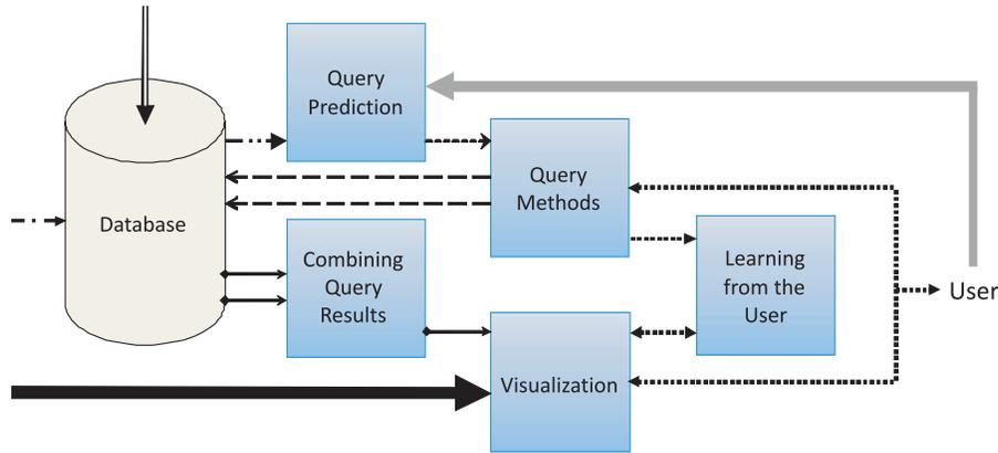
Fig. 3.1 General scheme for the retrieval frontend of a concept-based video search engine. Detail of Figure 1.3, building upon the conventions introduced in Figure 1.2. The scheme serves as the blueprint for the organization of this section.
