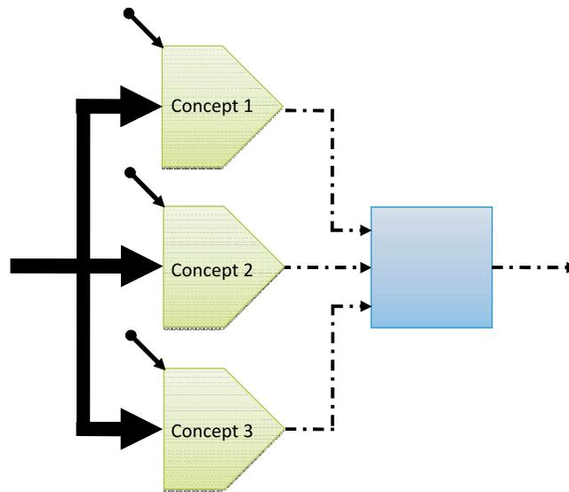
Fig. 2.5 General scheme for modeling relations between concept detectors. Outputs of multiple concept detectors are combined to improve existing detectors or to infer new concepts.
