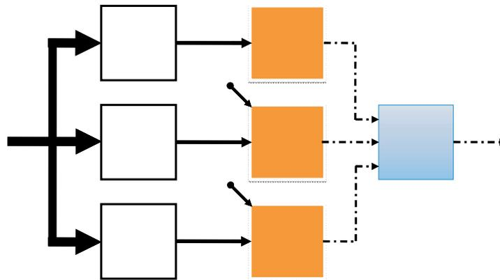
Fig. 2.4 General scheme for classifier fusion. Output of feature extraction is used to learn separate probabilities for a single concept. After combination a final probability is obtained for the concept, special case of Figure 2.2.
