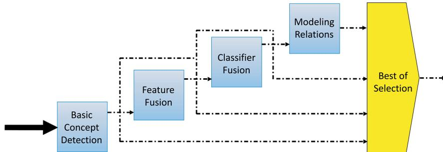
Fig. 2.1 General scheme for generic concept detection in video. Detail of Figure 1.3, using the conventions of Figure 1.2. The scheme serves as the blueprint for the organization of this section.
