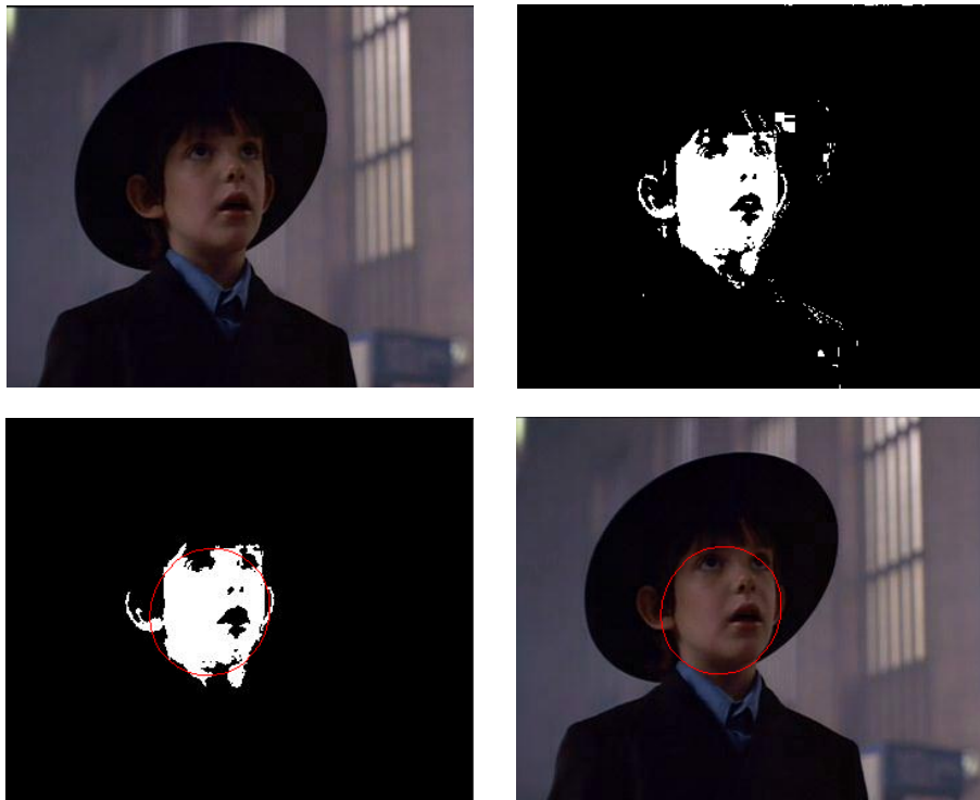
Figure 4.3: Top left: the original video frame; Top right: the frame after skin color segmentation; Bottom left: the frame after connected component and shape analysis; Bottom right: frame with detected face;
