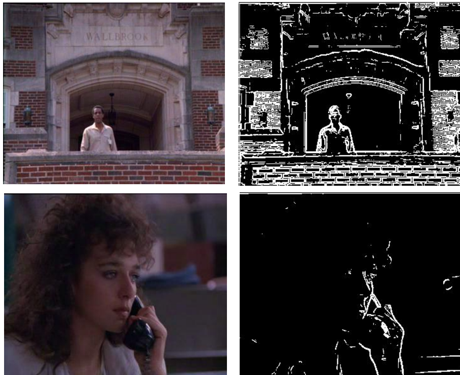
Figure 4.6: Top: a long shot with complex patterned background resulting in 22915 detected edge pixels out of 101376; Bottom: a close-up with smooth background resulting in 2490 detected edge pixels. Note that the foreground object also generates few edge pixels
