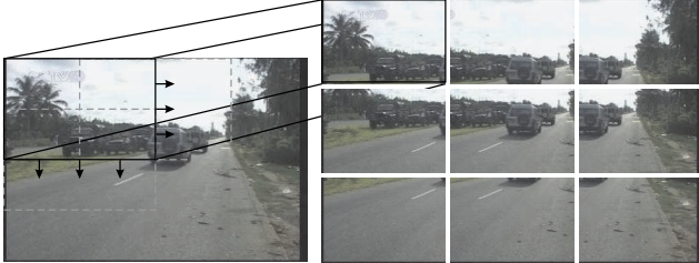
Figure 3. An example of dividing an image up in overlapping regions. Here, the region size is a \frac{1}{2} of the image size for both the x- and y-dimension. The regions are uniformly sampled across the image with a step size of half a region. Sampling in this manner identifies nine overlapping regions.
