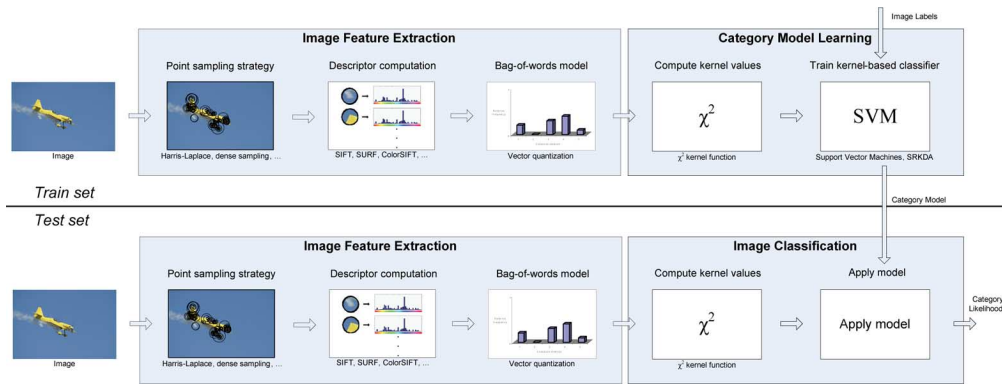
Fig. 1. Components of a state-of-the-art visual categorization system. For all images in both the train set and the test set, visual features are extracted in a number of steps. First, a point sampling method is applied to the image. Then, for every point, a descriptor is computed over the area around the point. All the descriptors of an image are subsequently vector quantized against a codebook of prototypical descriptors. This results in a fixed-length feature vector representing the image. Next, the visual categorization system is trained based on the feature vectors of all training images and their category labels. To learn kernel-based classifiers, similarities between training images are needed. These similarities are computed using a kernel function. To apply a trained model to test images, the kernel function values are also needed. Given these values between a test image and the images in the train set, the category models are applied and category likelihoods are obtained.
