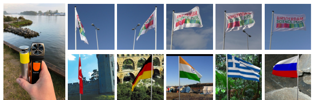
Figure 6. Left: Two anemometers used for gauging the wind speed. Right top: Real flag recordings with corresponding wind speeds measured by the anemometer hoisted in the flagpole. Right bottom: simulated examples from our FlagSim dataset.
